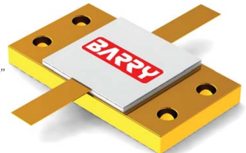
Rated Power: 800W Substrate: BeO Flange: Au Plated CuW Footprint: 1.900" x 1.040"
