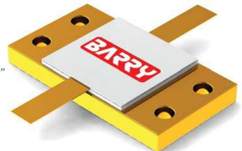
Rated Power: 800W Substrate: BeO Flange: Au Plated CuW Footprint: 1.900" x 1.040"
