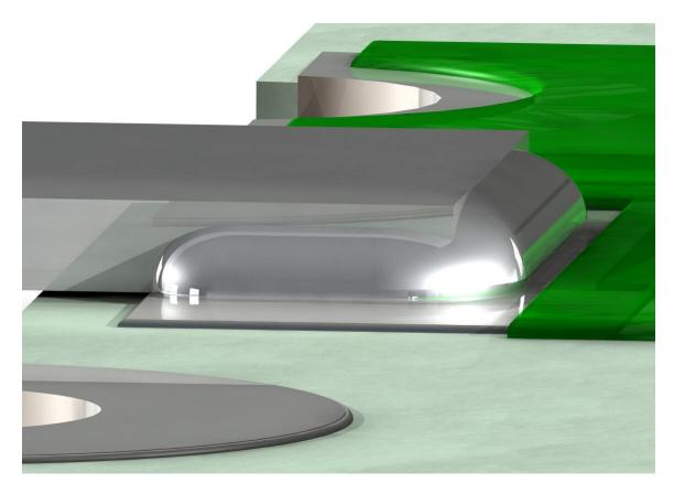
The rendering above depicts a typical lead attachment to a Barry "CT" chip. Notice that the fillet appears generally smooth and exhibits good wetting. There is good feathering or blending of the solder fillet to the areas of attachment, as well. This joint appears "bright" in nature but for customers using non-leaded solders IPC-A-610 does allow for some "dullness" or "graininess" to the joint, provided the joint is not "cold."
