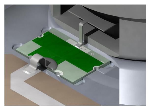
Notice in the above illustration that the customer is soldering a Barry Industries leaded device down, while attaching the lead from the output side to a circuit board and attaching a lead to the input side of the chip, all at the same time. The solder fillets are minimal, well within the bounds of the input pad and have a fillet shape in accordance with IPC-A-610.
